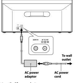
• Use the Sony supplied AC power adaptor only. The polarity of the plugs of other manufactures may be different. Failure to use the
